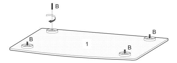
Carefully lay glass top (1) upside down on a soft surface. Screw short rods (B) into the metal plates of glass top (1).
